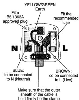
the terminals in your plug, proceed as follows: The wires that is coloured Brown must be connected to the terminal which is marked with the letter L or coloured Red. The wire that is coloured Blue must be connected to the terminal which is marked with the letter N or coloured Black.
